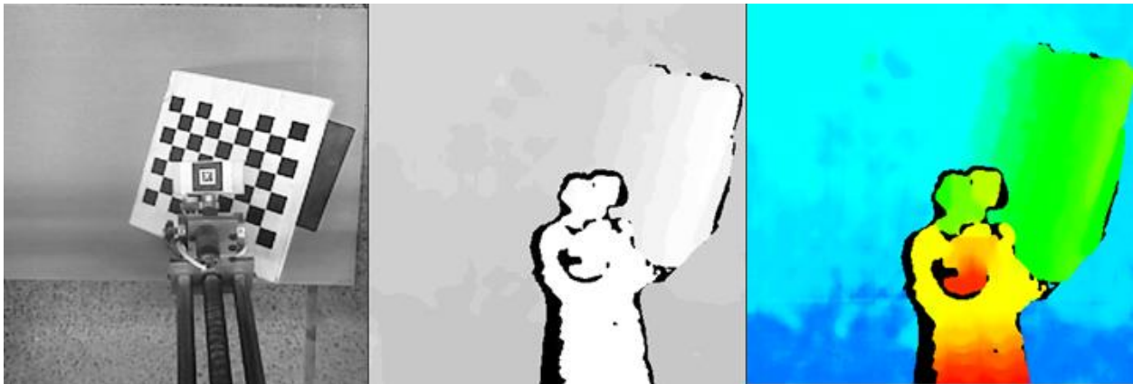
Figure 15. Scene image, its corresponding disparity map, and its 3D point cloud
