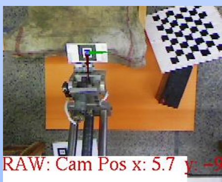
Visual feedback for end-effector 3D pose detection (ARToolkit)
