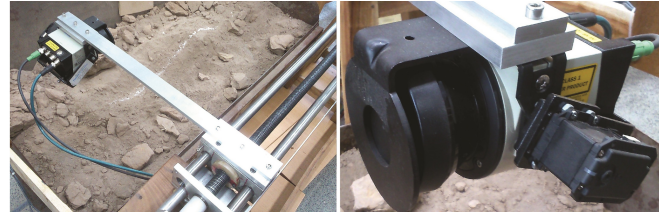
Fig. 6. Hardware assembly of scaled lab model with scanner maneuvering above along canal length axis (left). Close-up of LMS151 scanner (right).
