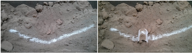
Fig. 9. Two states of the channel model: (a) Baseline (left); (b) Silted (right).
